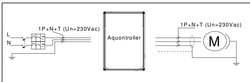
\* Power cable section according to length with a 1.5kW electric pump.
